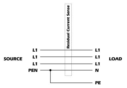
Due to the required installation of the functional earth, upstream protection by Residual Current Protective Devices will not be possible, as they will malfunction due to the leakage current from the UPS.
